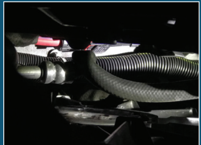
Example of twisted cooler line
