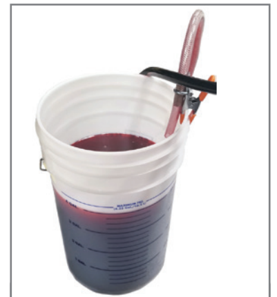
Use the DT-52263 Transmission Fluid Exchange Kit to perform the fluid exchange.
